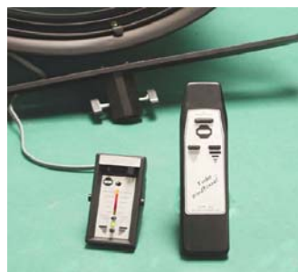
Model 1000 infra-red remote control and detachable control panel with LED speed indicator.
